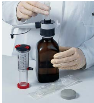
Sterile dispensing cartridge installation
