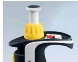
Red recalibration flag indicates adjustment from factory specifications.
