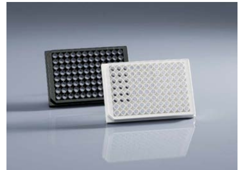
96-well transparent bottom microplates
